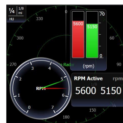
Analog gauge showing RPM from two engines.
